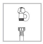
1. Connect the inlet hose by screwing it to a cold water tap using a 3/4 gas threaded connection (see fiaure).
